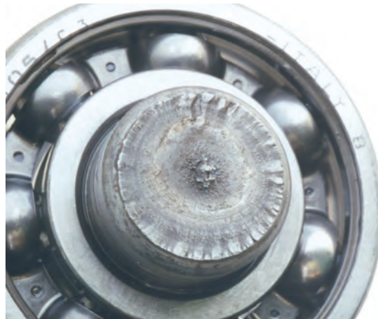
Rotational bending fatigue
